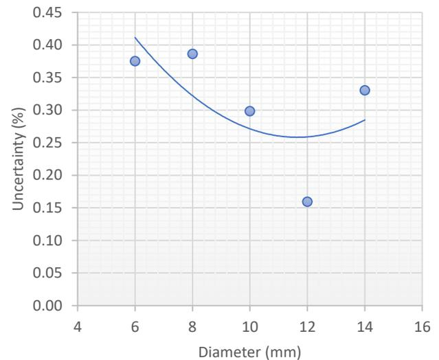
Figure 9 : Variations of uncertainty of reinforcing steel bars with their diameter - Section reduction.
