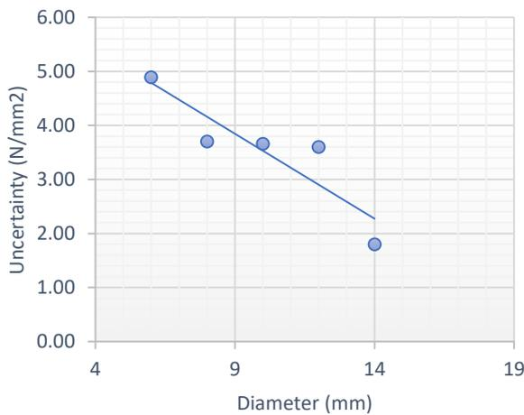
Figure 5 : Variations of uncertainty of reinforcing steel bars with their diameter - Ultimate Tensile Strength.
