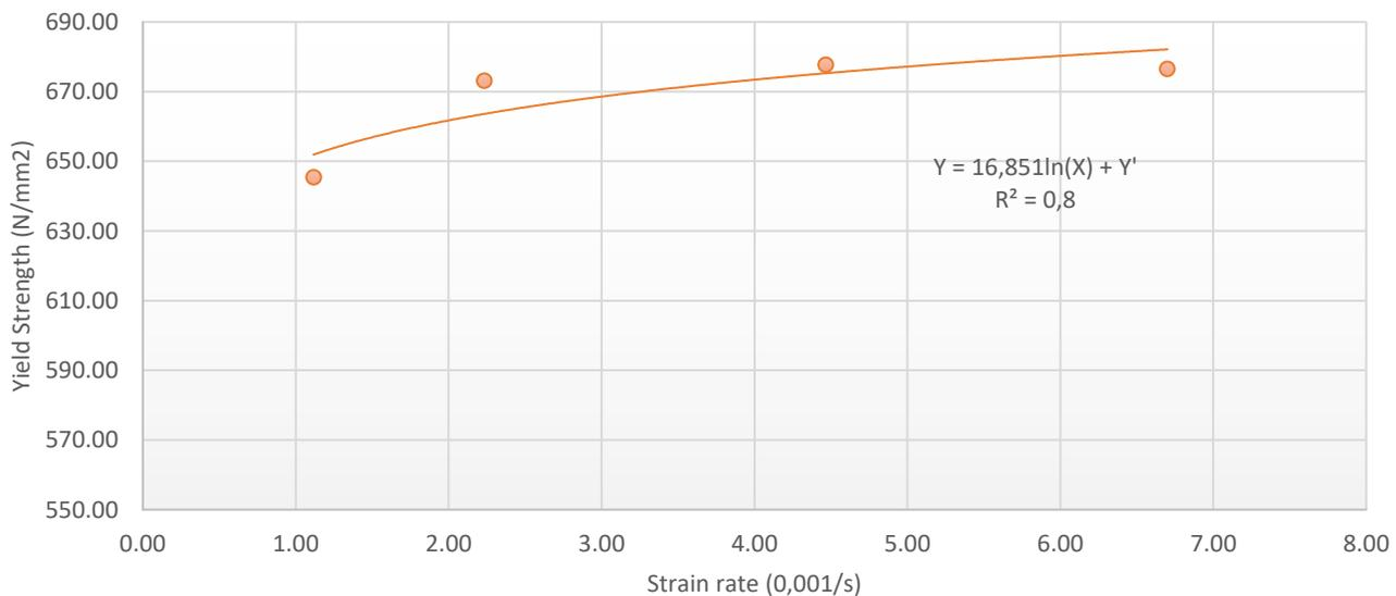
Figure 10 : Variations of Yield Strength of reinforcing steel bars with strain rate.
