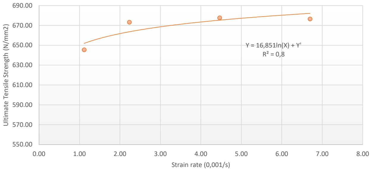
Figure 11 : Variations of Ultimate Tensile Strength of reinforcing steel bars with strain rate.
