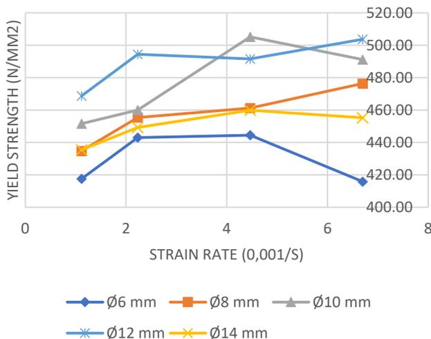
Figure 2 : Variations of yield strength of reinforcing steel bars with strain rate.
