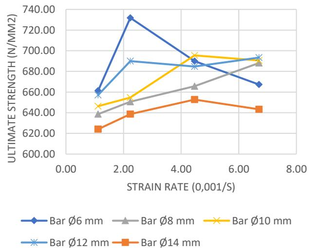
Figure 4 : Variations of ultimate tensile strength of reinforcing steel bars with strain rate.
