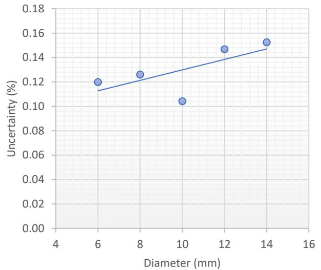
Figure 7 : Variations of uncertainty of reinforcing steel bars with their diameter - Elongation.
