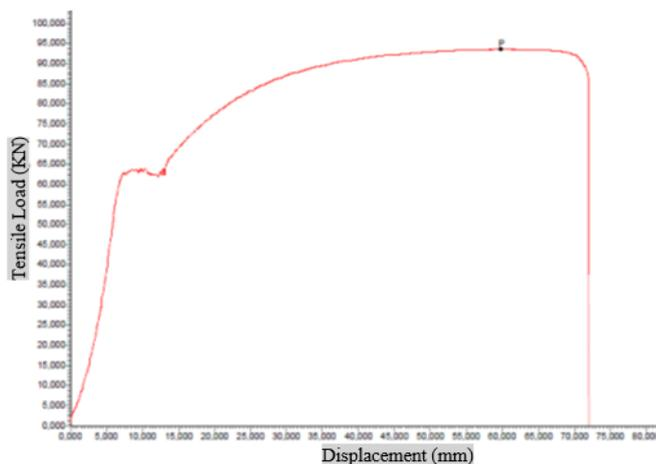
Figure 1 : Example of Data Recorded in Tensile Tests: Tensile load (KN) versus Displacement (mm)
