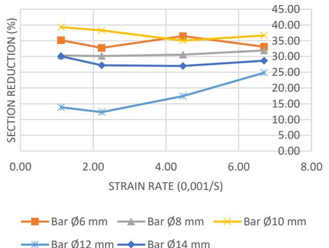
Figure 8 : Variations of section reduction of reinforcing steel bars with strain rate.
