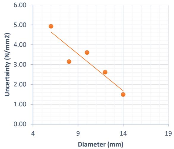
Figure 3 : Variations of uncertainty of reinforcing steel bars with their diameter – Yield Strength.
