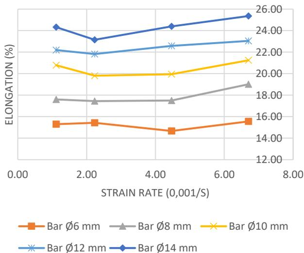
Figure 6 : Variations of elongation of reinforcing steel bars with strain rate.
